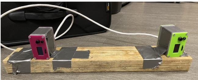
FIG. 4. Image of detectors secured onto wooden plank and connected by ethernet for coincidence counting.
