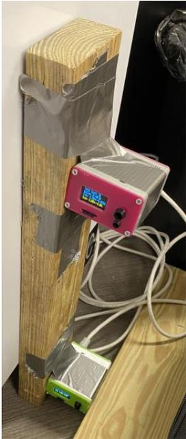
FIG. 8. Slight sag in top detector due to duct tape coming loose.
